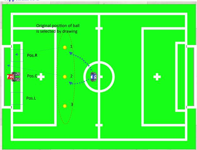
There is one of the 3 possible positions of the ball selected by a draw to free kick facing each position of the obstacle robot.
